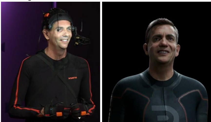
Figure 2-10: Doug Roble wears the motion-capture suit and camera (image on the left) that brings DigiDoug to life (image on the right). ©Digital Domain.
