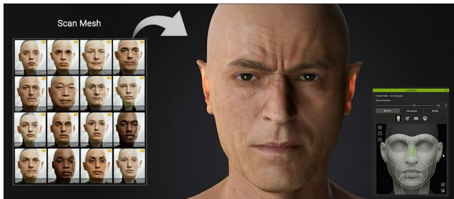
Figure 2-20: Mapping of a 3D Scan mesh of a head within Character Creator.
