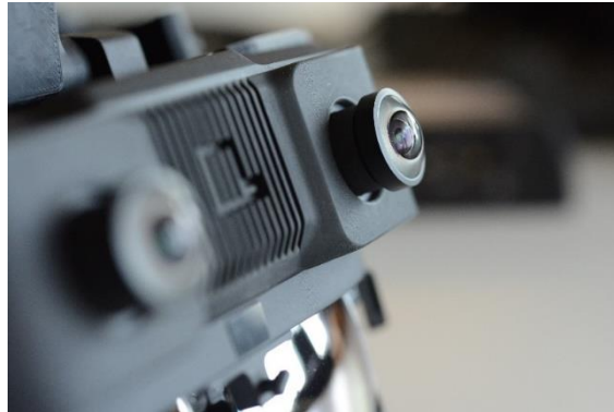
Figure 9. Fisheye lenses installed on a XR HMD V1 as used for the pose tracking and hand tracking tests.
