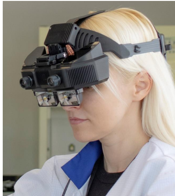
Figure 4. Multi-focal (4-focus planes) IG-1050 AR HMD by Lightspace.
