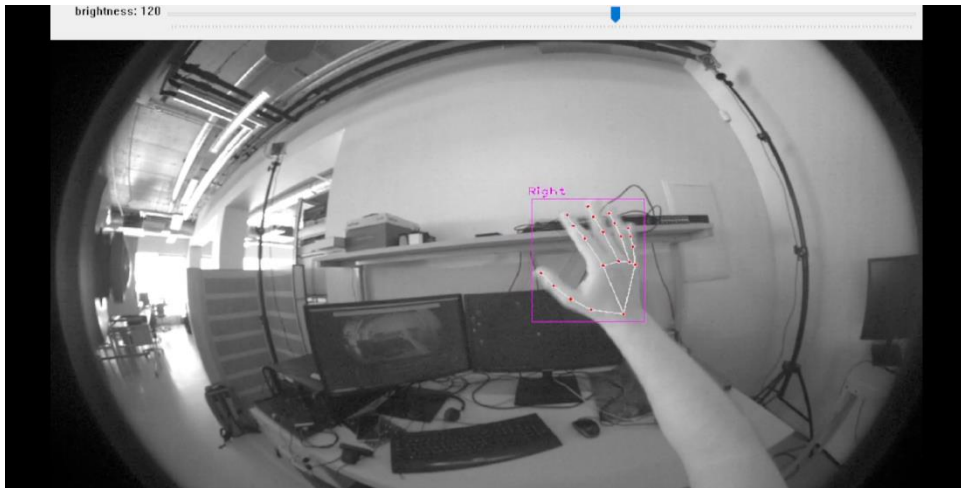
Figure 15. Actual view of a fisheye camera lens as used for hand tracking routines.
