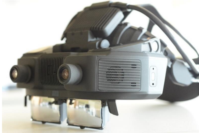
Figure 10. Appearance of a multi-focal HMD as used for the V1 demonstration.
