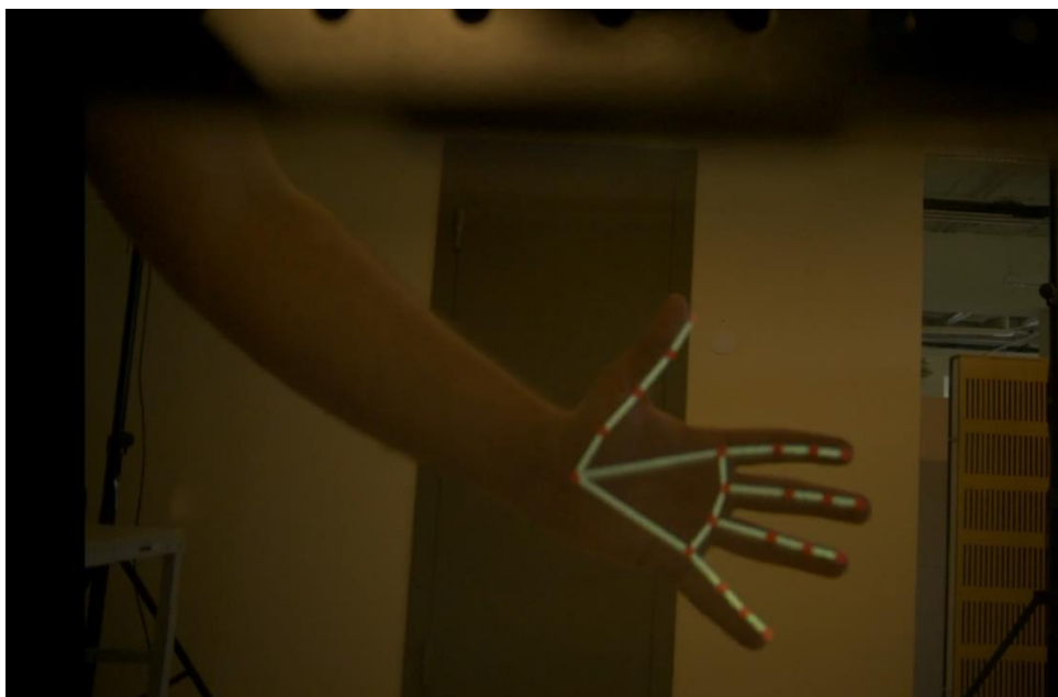
Figure 16. “Through-the-lens” capture of hand-tracking overlay as it can be seen through XR HMD.
