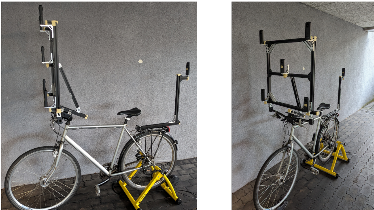
Figure 2 – Bicycle capturing rig with six Theta Z1 cameras from Ricoh.
