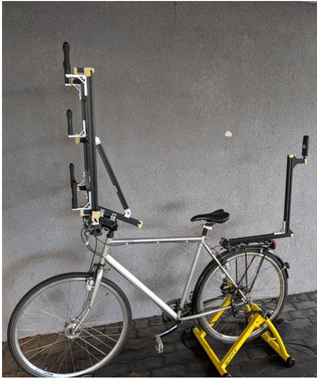
Figure 10 The camera rig with six cameras attached to a bicycle
